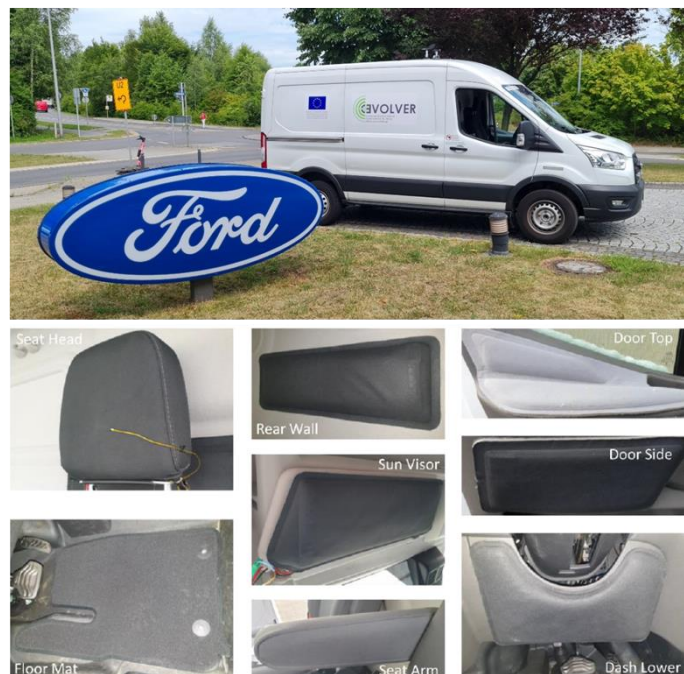
Figure 3-3: Ford delivery van and heating panels installed around the driver (Source: "Advanced Thermal Management"; Alexander Wahl, CEVOLVER Final Event, 2022-09-27, Aldenhoven Testing Center, Germany)
