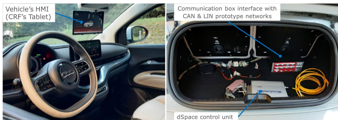
Figure 6-3: Connectivity and HMI features installed in CRF's Validator 2. (Source: "Long trip simulations and realisation Part 2"; Patrizio Turco, CEVOLVER Final Event, 2022-09-27, Aldenhoven Testing Center, Germany)
