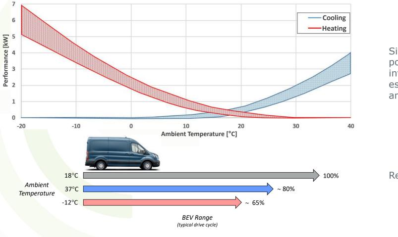
Significant amount of power required for interior climatization especially at cold ambient temperatures
