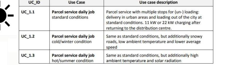
The impact of certain boundary conditions as ambient temperature and solar radiation have a high impact on low load cycles due to that fact the ratio between propulsion and interior climatization energy is unfavourable. Hence, these boundary conditions have been varied for the parcel delivery service usage scenario.
